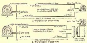
Fig. 133.—Advantage of high-voltage transmission.
